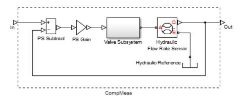
It represents a composite component CompMeas, which, in turn, contains a composite component Valve Subsystem, as well as several Foundation library blocks. The Simscape file of the composite component would specify the equivalent signal connections with the following constructs.
