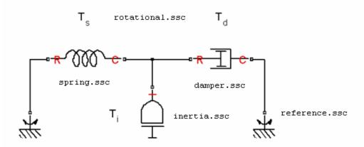
The domain is declared in a file named rotational.ssc (see "Declare a Mechanical Rotational Domain" on page 2-13). The following file, named spring.ssc, declares a component called spring. The component contains:
