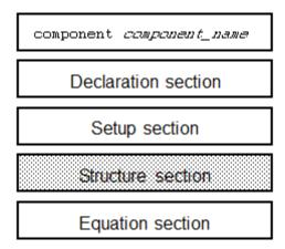
The structure section begins with a connections keyword and is terminated by an end keyword. This connections block contains a set of connect constructs, which describe both the conserving connections (between nodes) and the physical signal connections (between the inputs and outputs).
